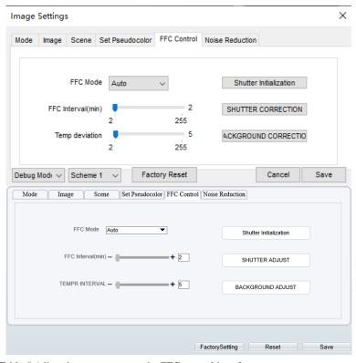
Figure 5-7 FFC Control Interface
