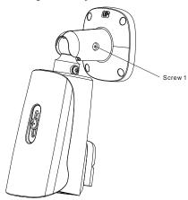
Step 3 Install the camera on the ceiling or wall and fixe the screws as shown in Figure 1-3. Figure 1-3 Fix Camera
