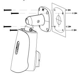
Step 4 Connect the multi-connector cable and monitor, loosen the screw 2 to adjust the position so that the camera face the monitored area, as shown in Figure 1-4. Tighten the screw 1 and screw 2.
