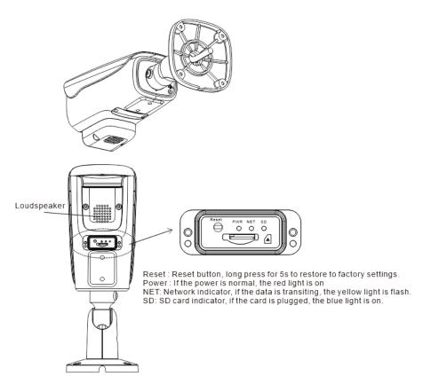
Reset: Reset button, long press for 5s to restore to factory settings.
