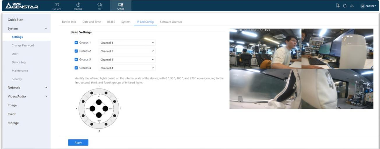
The IR led is corresponded as the figure on page. Identify the infrared lights based on the internal scale of the device, with 0°, 90°, 180°, and 270° corresponding to the first, second, third, and fourth groups of infrared lights. The position is marking on the device, users should make sure the position before installing.
