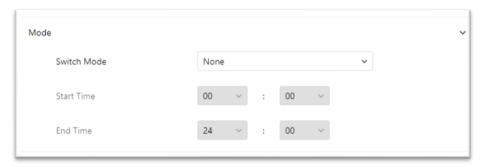
Step 2 Choose Switch Mode, there are three modes to be chosen, none, time mode, D/N linkage mode.
